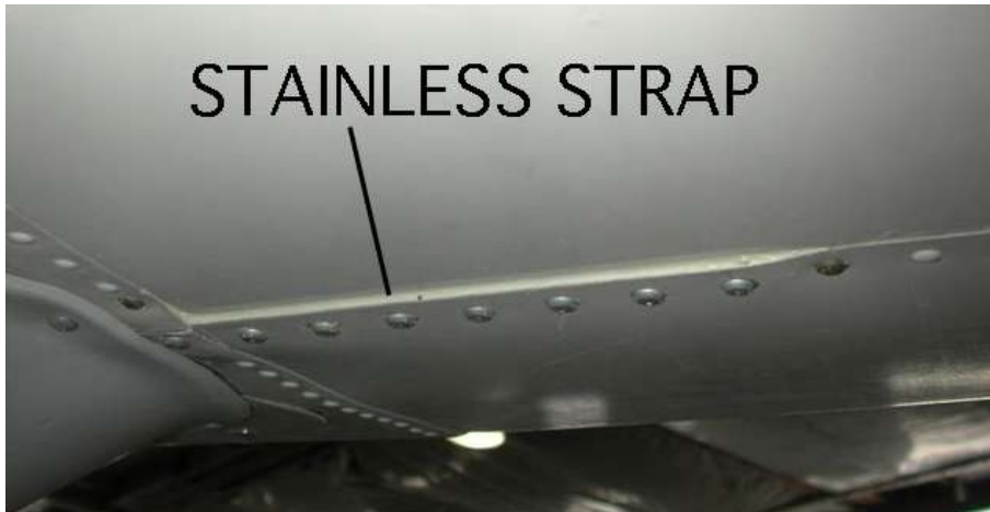
Fig 3: Stainless Strap (under leading edge skin at wing station 100) RH Wing shown, looking forward Refer to Air Research Technology Inc. Wing Extension and Spar Reinforcement Installation Guide #172 Part III for applicability of this reinforcement to your aircraft.
